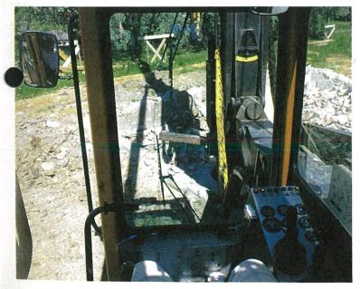
By siting controls alongside the operators seat excellent forward visibility of the work area is achieved. Inclinometers indicate the rake of the leader in two planes. The FOPS standard cab is acoustically isolated and vibration damped to the highest specification and is fully enclosed in a steel safety cage.
