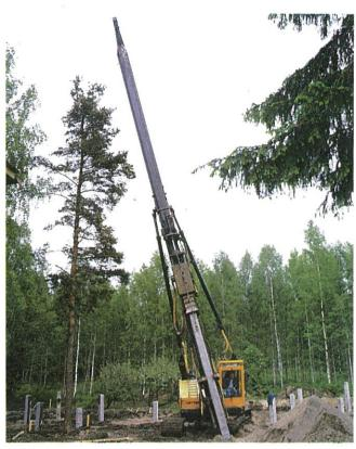
Crawler spread and counterweight width provide an extremely stable undercarriage permitting pile driving over the widest possible range of inclined angles.
