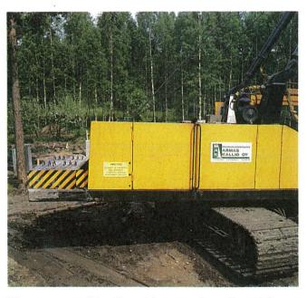
The counterweight disposition may be adjusted by up to 1 metre directly from the operators cab and the amount of counterweight be changed by adding or removing modular sections.
